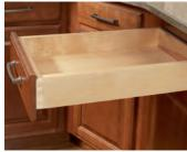
5%" Plywood dovetail drawer box in natural finish with laminated plywood drawer bottom and undermount soft close drawer slides. Dovetail joints are unfinished.
