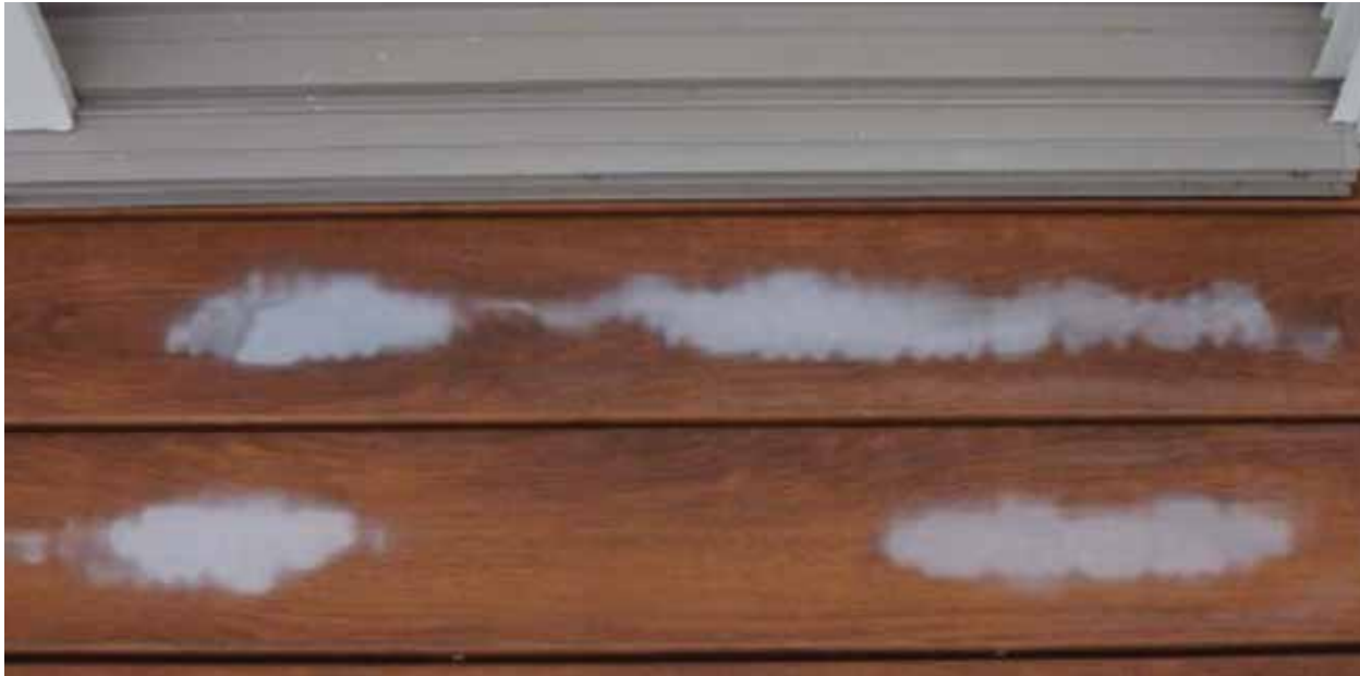
Example of discoloration that can be caused by using these products on Zuri® Deck.
