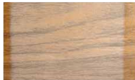
Sample 2 NOT Protected with Acrylic Topcoat 11.62 delta-E color change
