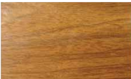
Sample 1 Protected with Acrylic Topcoat .78 delta-E color change
